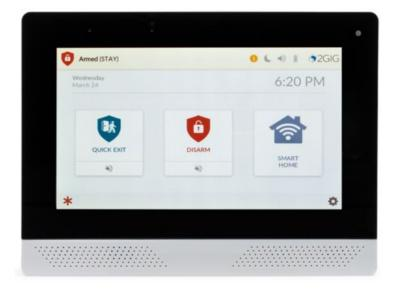
• If there are unacknowledged trouble conditions, the header bar flashes orange and a numeric icon will display how many unacknowledged conditions exist. Tap the numeric icon, then tap "Alerts" to view the trouble conditions.
