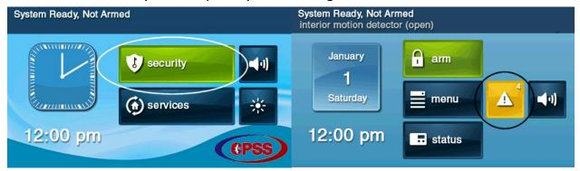
• Use the up/down arrows to scroll through the alerts to clear them, then press *Ok* to exit. This action will silence the beeping for 4 hours, but the issue must be resolved in order for beeping to completely end, and clear alerts for issues that have been resolved.
